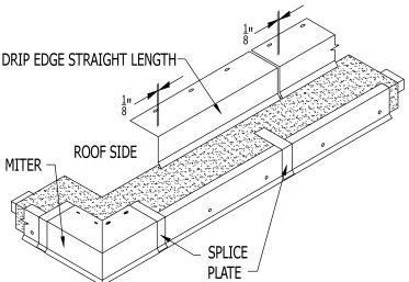
**STEP 4**: Installing Drip Edge Straight Lengths
