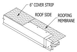
**STEP 5: Installing Approved Roofing Membrane**Install 6" Cover Strip per roofing manufacturer's instructions.
