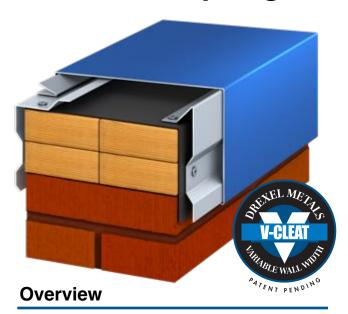
JAMF Spring-Tite Coping EZ system is a two-part assembly that includes a front and rear segmented cleat and a decorative snap-on coping cover for single ply commercial roof systems.
