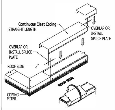
**STEP 3:** Installing Continuous Cleat Coping Straight Lengths
