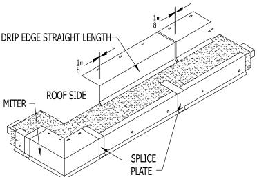
**STEP 4**: Installing Drip Edge Straight Lengths
