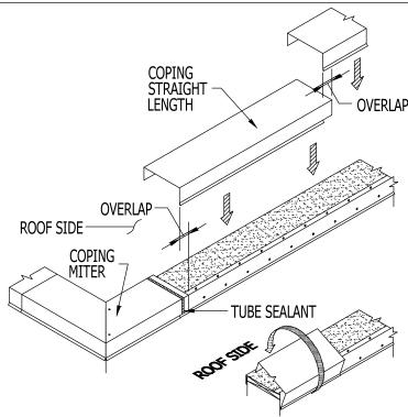
Start by notching the end of the Coping opposite of the installed Miter. Apply a bead of Tube Sealant. Install the Coping by hooking the drip over the kick out on the Cleat and rotating the Coping over the parapet wall and screw the roof side leg of the coping with #9-13x1-1/2" S.S. Washered Screws provided at 12" on center. Consider lengths of all straight pieces prior to cutting to avoid creating relatively short sections adjacent to one another.
