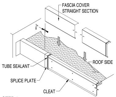
**STEP 4:** Installing Fascia Cover Straight Lengths
