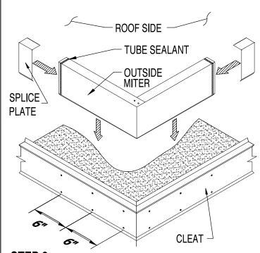
STEP 2 : Installing Fascia Cover Miters
