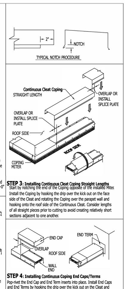
be restrained from moving by securing with a minimum of (2) #10-13x1" S.S. Panhead Woodscrews through the roof side leg.
