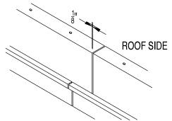
STEP 5 : Installing Gutter LT Straight Lengths
