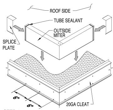
STEP 2 : Installing Fascia Cover Miters
